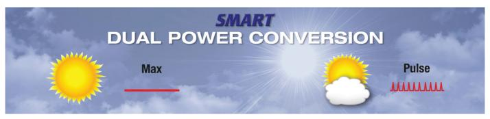
The OptiMate charge controller adapts to the available power that the solar panel can provide and adjusts it to efficiently charge the battery. The controller automatically varies it's charge rate between continuous charge at full sun and pulse charge at low light. This dual method of charging ensures that even during low light the battery will receive high current pulses of energy.
